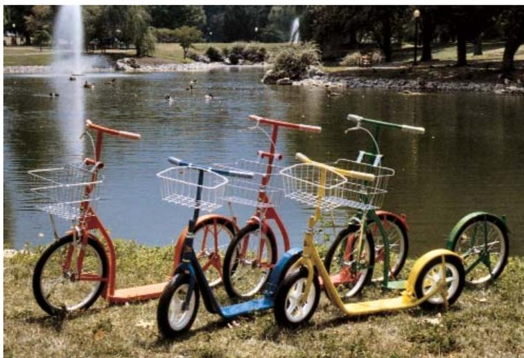
Made on a local Amish farm, these scooters feature welded steel construction, ball bearing wheels, high speed aluminum racing rims, standard bicycle pneumatic tire sizes, powder-coat finish, front and rear brakes, kick-stand, bell, and a front basket.
